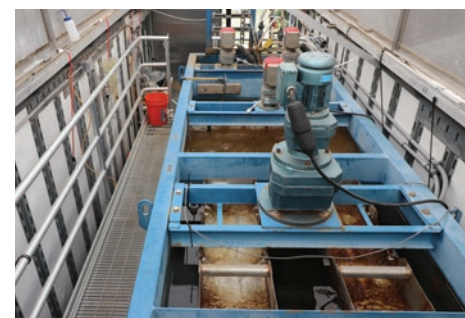
The pilot unit is trailer mounted and includes a full laboratory and remote-operation capabilities.
