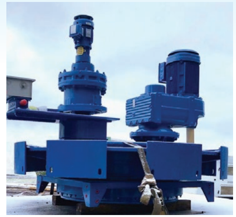
WesTech's dual-cage retrofit bolted seamlessly into the allotted space.
